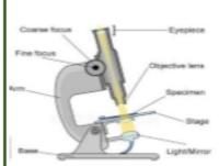
Light Microscope: A device which uses light and a series of lenses to produce a magnified image of an object.
